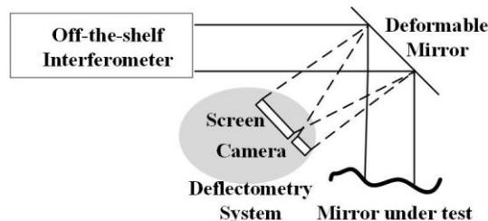
Fig. 1. Schematic of the proposed adaptive interferometric null system, with the three subsystems: Interferometer, deflectometry system and deformable mirror. [4]
