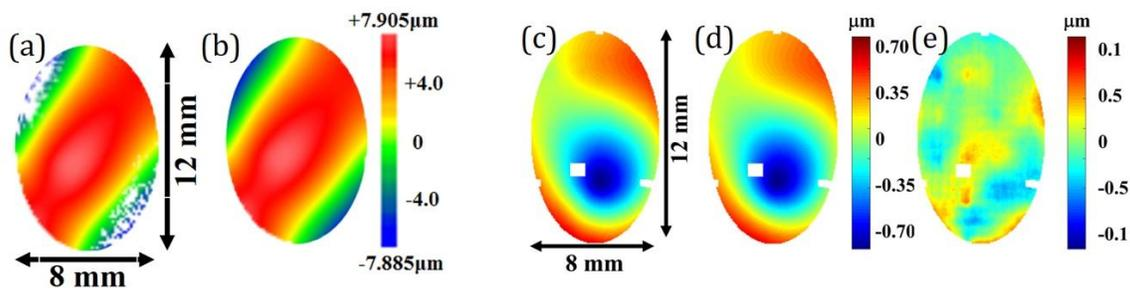
Fig. 3. (a) The initial interferometric measurement which does not cover the entire area due to standard interferometer's limited dynamic range. (b) Final surface map based on data obtained by the proposed adaptive interferometric system. (c) Checking the validity; adaptive interferometric measurement (d) Checking the validity; standard interferometric method (e) Difference map of (c) and (d). [4]
