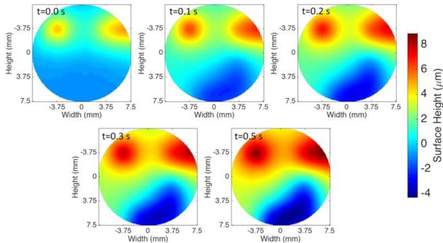
Fig. 5. Measured surface evolution (as a function of time) of the deformable mirror, where a set of actuators are moving linearly together from lower voltage to higher voltage.
