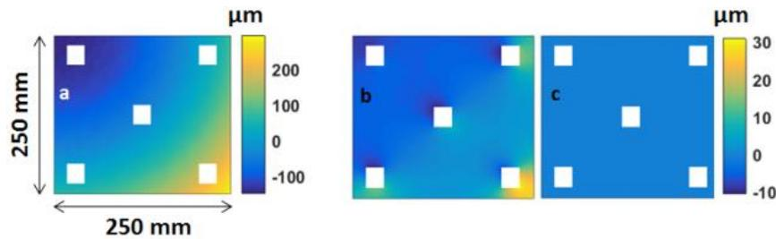
Fig. 6. (a) Simulated ideal surface data with 5 fiducial masks. (b) Southwell and (c) modal residual error maps (differences between the reconstructed surface map and the simulated ideal map).
