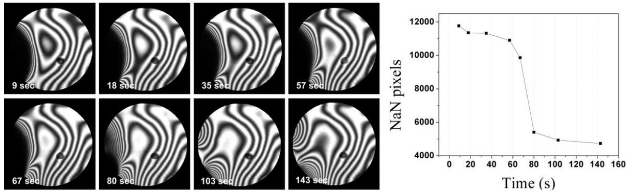
Fig. 2. Time evolution characteristics of a SPGD-guided fringe restoration process along with change in evaluation criteria that guides the process.
