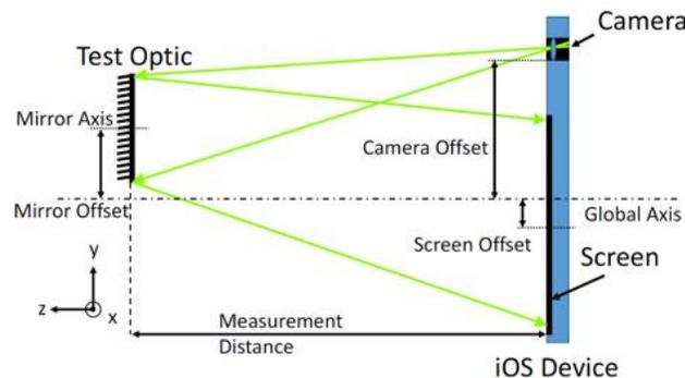
Fig. 4. A schematic of the proposed instantaneous phase shifting deflectometry system using iPhone's camera and screen. [5]
