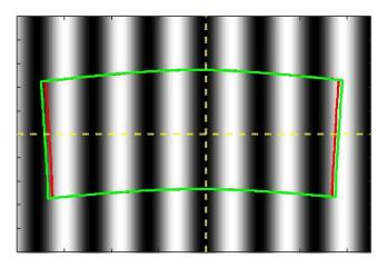
Figure 4. Effective area of screen when perturb the UUT with translation in X (red outline) and tilt in Y (green outline). The position of effective area is similar, but different in size especially in horizontal direction.
