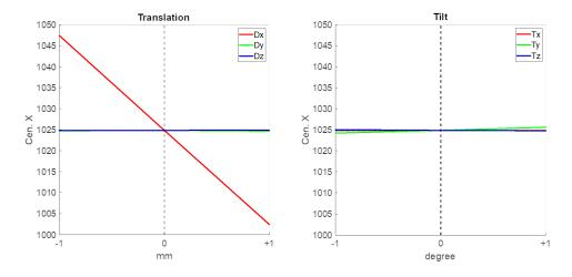
Figure 6. Sensitivity trend plots of X-centroid for all misalignment cases. Translation in X shows most sensitivity, and other misalignments have negligible slopes.
