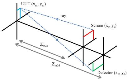
Figure 1. Simple diagram of a deflectometry system.<sup>5</sup> The path of a single ray traced in the deflectometry system. To obtain local slope of UUT, we need the coordinates of screen pixel ( $x_{s}$ ,  $y_{s}$ ), detector pixel ( $x_{d}$ ,  $y_{d}$ ), sampled position ( $x_{m}$ ,  $y_{m}$ ), and distances along the optical axis from UUT to screen and detector,  $Z_{m2s}$ ,  $Z_{m2d}$ .
