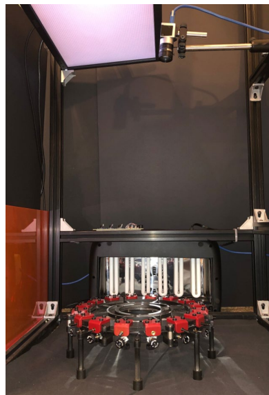
Figure 7. The deflectometry measurement system consisting of the KEYS (bottom), a screen with modulated sinusoidal pattern image (upper left) and a camera (upper center) to capture the reflection off the MODE lens segment surface.
