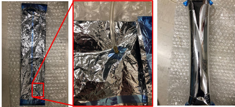
Figure 5. The photos of the pillow sample. (left) the adhesion and seamed area are taped. The red box represents the air inlet position. While optical testing, the inlet, and seamed area face downside. (middle) Air inlet. (right) Fully inflated pillow. At the middle of the pillow, the crease removal upon pressurization to a stress level below the membrane's yield point and adhesion area puncture.
