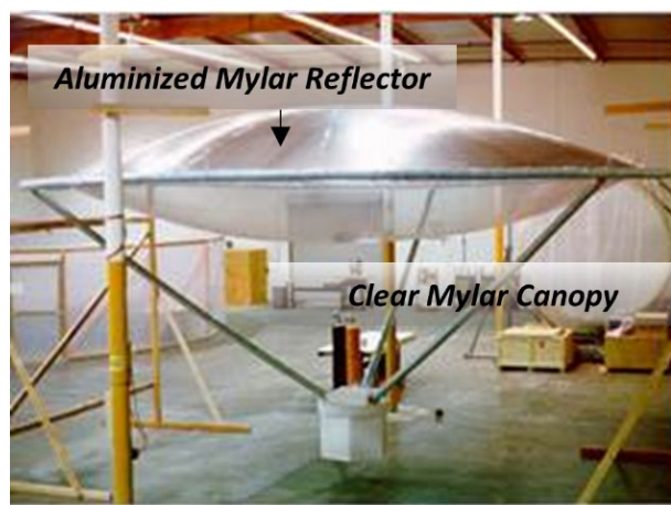
Figure 2. Prototyping 7 m diameter inflatable reflector in L’Garde site. The lenticular structure consists of the aluminized reflector and symmetric canopy.
