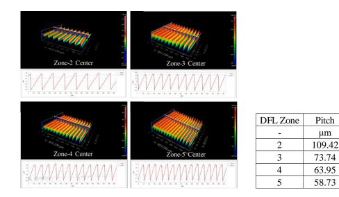
Figure 4. Single-harmonic DFL profiles measurement using Zygo NewView 3D optical surface prolier
