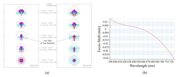
Figure 2. Performance of prototype MODE lens telescope. (a) Spot diagram within Airy disk of 6.7μm, where left is spots for design telescope lens and right is spots for the telescope with a fabrication error of a color corrector.
