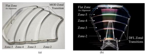
Figure 3. Prototype molded ring segment. (a) High-harmonic MOD zones and (b) Single-harmonic DFL zones
