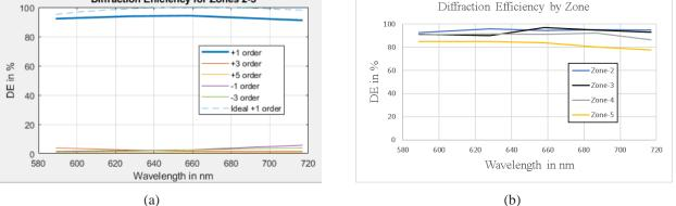
Figure 5. Measured diffraction efficiency (DE) of the test molded ring segment. The +1 order is the design order. (a) Diffraction efficiency over all wavelengths averaged for zone 2-5 and (b) Diffraction efficiency by zone 2-5 for the +1 design order.
