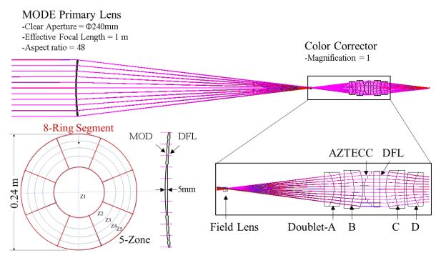
Figure 1. Prototype MODE lens telescope with color corrector
