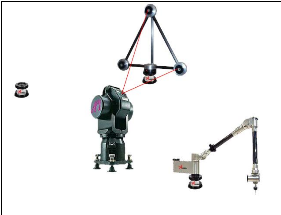
Figure 2.10. Combining a Laser Tracker with Coordinate Measuring Arms. [35]
