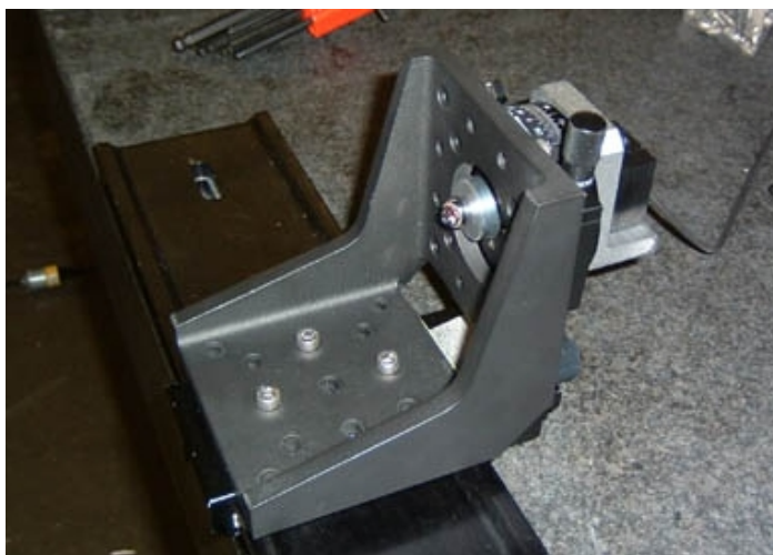
Figure 3.35. PSD/Tracker Ball Assembly mounted on Rail
