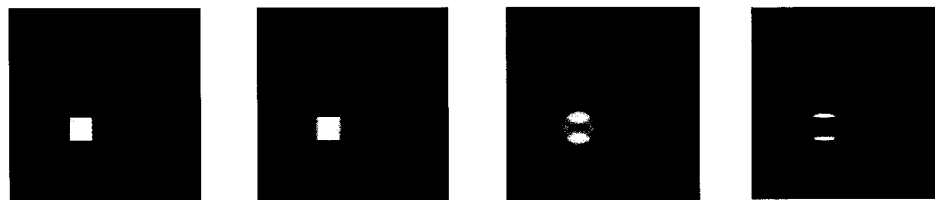
FIGURE 3.6. Degradation when limiting the measurement angle. From left to right we have a total view angle of 180^\circ , 120^\circ , 60^\circ , 20^\circ .
