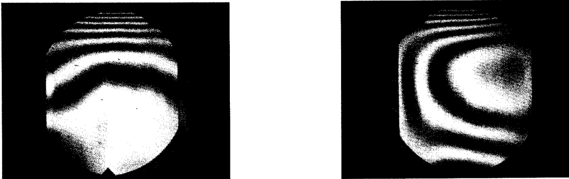
FIGURE 4.5. Interferogram at left has been rotated 15^\circ clockwise from where the face is perpendicular to the interferometer. At right, the interferogram has been rotated 14^\circ counter-clockwise.
