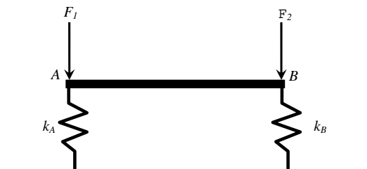
Figure 7.2: First configuration of forces examined for the rod and spring system example. Force one pushes on the rod directly over point A and force two pushes on the rod directly over point B .
