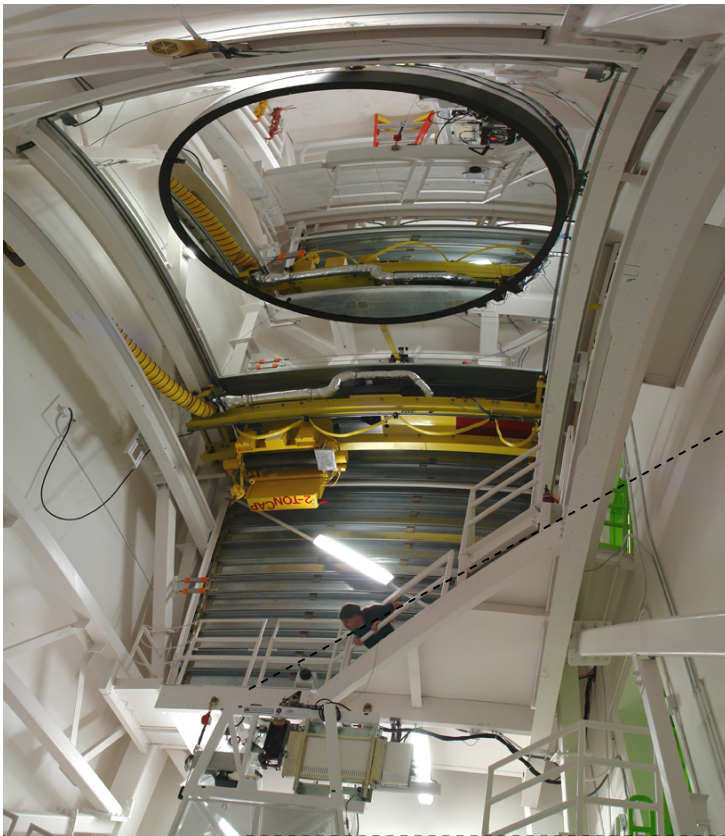
Figure 4. Shaping of the wavefront by the null corrector. The interferometer's spherical wavefront is shaped first by the CGH, then by the 76 cm sphere, and finally by the 3.75 m sphere.
