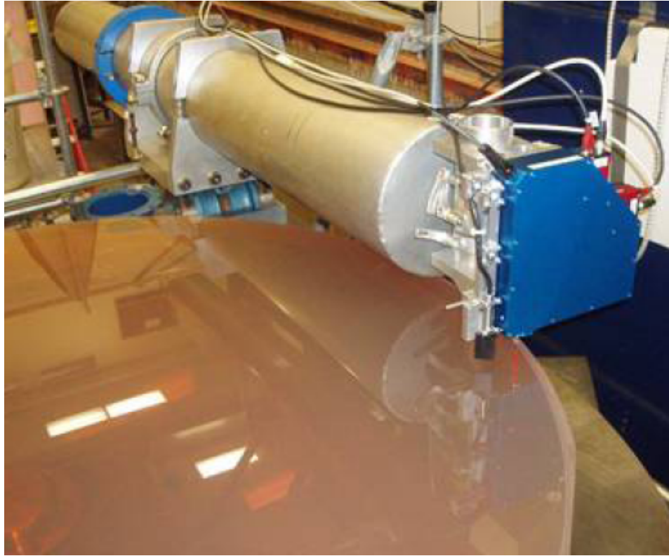
Figure 9. Photograph showing the SOCMM in use over a convex, off axis asphere (1.5 m diameter).
