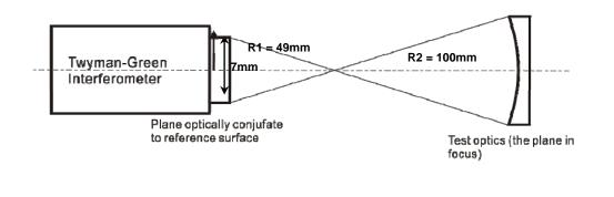
$$L_e = \frac{R_1(R_1 - R_2)}{R_2} = \frac{49 \cdot (49 + 100)}{-100} = -73 \text{mm}$$
