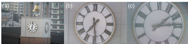
Fig. 12. TRT kit field test pictures. The pictures were captured with the (a) Newtonian, (b) Cassegrain, and (c) Gregorian telescopes, respectively. Each telescope has a different FOV, and the picture with the Gregorian telescope is reversed.
