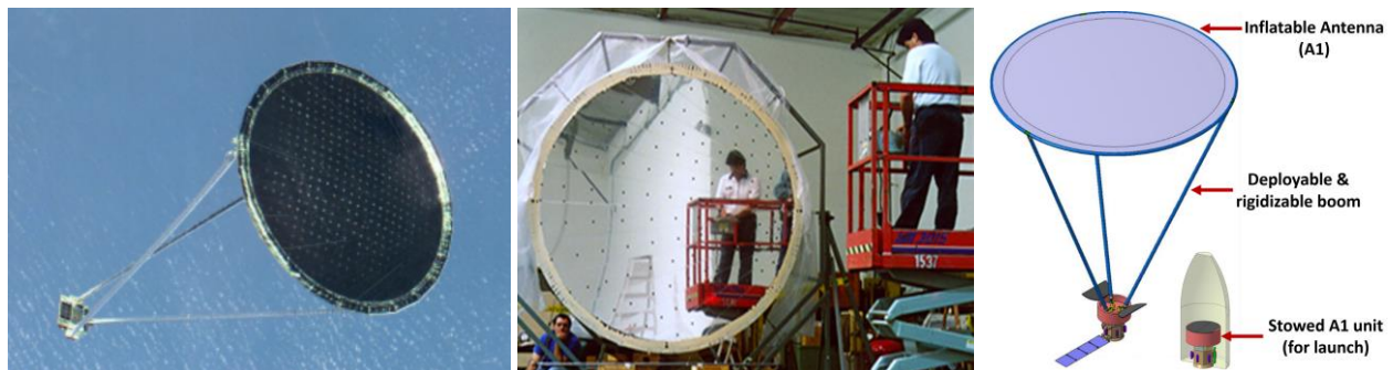
Fig. 1. Left: 14-m diameter IAE (Inflatable Antenna Experiment) system during the test operations in space with the Space Shuttle Endeavour . [3] This inflatable antenna designed and manufactured at L'Garde in 1997 is the predecessor of SALTUS, which is a mid/far-infrared telescope concept utilizing an advanced 20-m scale inflatable mirror antenna. Middle: 5-m diameter off-axis subsector of the IAE undergoing photogrammetry testing at the L'Garde facility. The “dots” are retro-reflective targets for photogrammetry. The measured surface accuracy of this predecessor antenna was already achieving ~0.32 mm RMS relative to the best-fit parabolic surface. Right: SALTUS/OASIS deployable architecture enabling stowed configuration for launch and deployed-and-inflated telescope in space. [1]
