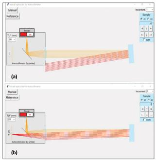
Fig. 2. Screen capture of a virtual lab focusing on optical surface alignment with an autocollimator. (a and b) The failure-mode-enabled case (a) shows large misalignment errors when compared to the nominal case (b). The disk (blue) is the unit under alignment and the incoming beam (orange) and reflected beam (red) are used for measurements of the surface.
