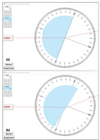
Fig. 1. Screen capture of a virtual lab illustrating the index of refraction of the glass block (blue) and Snell's law of refraction measurements. Examples show a nominal setup (top) and a failure-mode case (bottom). Movement of the rotating disk and the glass block are controlled from the top-left corner of the virtual lab panel.
