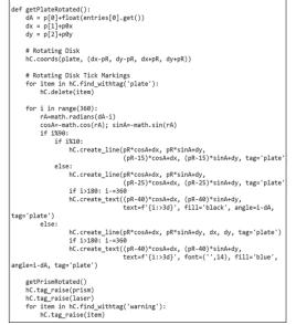
Fig. 3. A segment of the open-source Python script used for the Snell's law virtual lab shown in Fig. 1. This segment of the script defines the rotating protractor disk measuring the angle of the ray.
