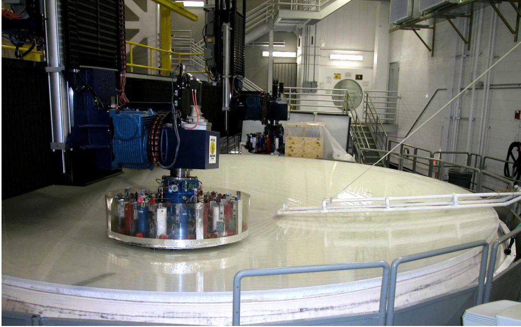
Figure 4. The Mirror Lab's 8.4 m capacity Large Polishing Machine, shown with the second LBT primary mirror. With two carriages, the machine can be used with a variety of actively stressed laps and passive tools. The photo shows two 1.2 m stressed laps.
