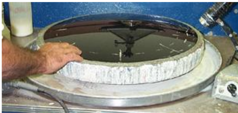
Figure 8. The glass fabrication process. A: The concave optical surface is figured while the mirror is still a thick, stiff blank. B: We create a stiff blocking body. C: The glass is attached to the blocking body using pitch. D: All of the excess glass is removed. E: The glass is removed from the blocking body.
