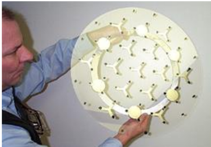
Figure 13. Finished glass, 0.5-m in diameter and 1 mm thick. The ring is just a handling fixture – it is not part of the finished mirror.
