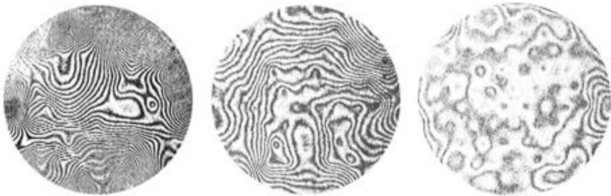
Figure 15. A progression of interferograms. Left: The initial measurement. Middle, Right: By manipulating the actuators, we can correct the figure. The middle figure shows 2 wvs surface rms, and the figure on the right shows 0.5 wvs surface rms (HeNe).
