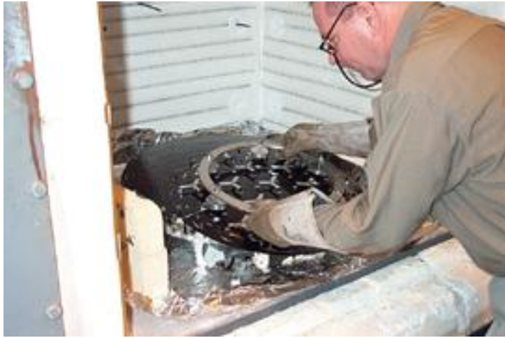
Figure 12. Steve Miller removes the thin shell from the granite blocking body.
