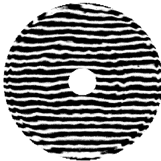
Figure 18. Interferogram at 633 nm calculated from the final data shown in Fig. 17.
