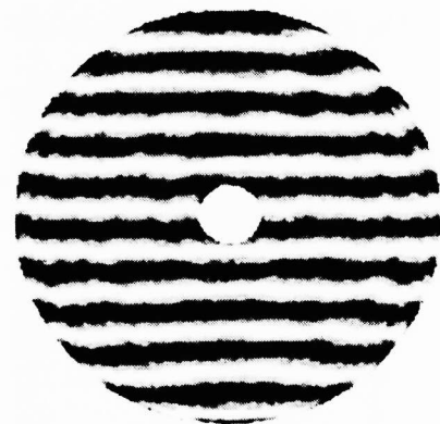
Figure 10. Interferogram, calculated from measurements for \lambda = 1 \mu\text{m} , showing the figure of the 6.5-m primary.
