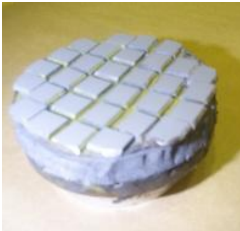
Figure 8. Composite tool with grinding tiles, plastic membrane, neoprene foam, and rigid backing plate.
