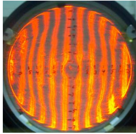
Figure 11. Measurement of the lens in Fig. 10 after 5 hours of work with the membrane tool.
