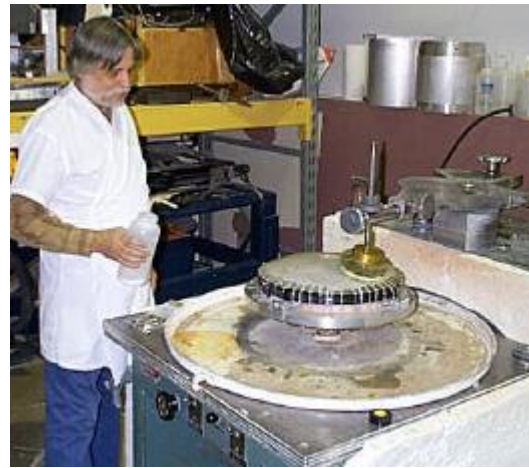
Figure 9. The membrane tools were run using conventional polishing machines.
