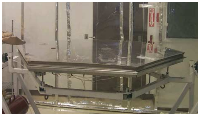
Figure 17. NMSD glass shell resting on vacuum support tool.
