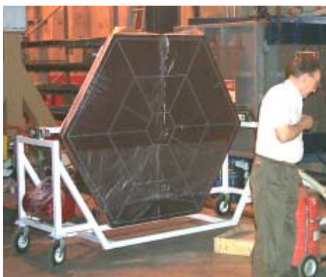
Figure 16. Vacuum support tool and handling cart
