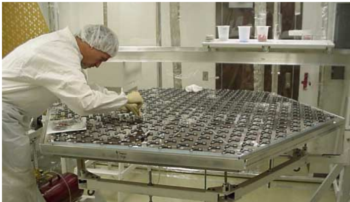
Figure 20. NMSD glass with pucks and sub-loadspreaders.
