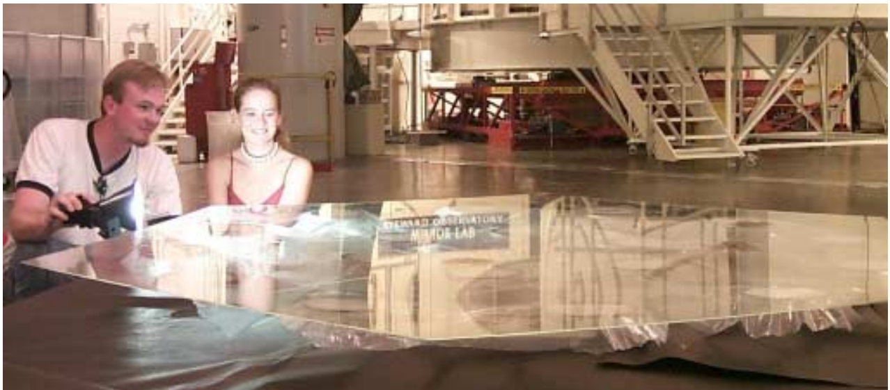
Figure 15. Completed 2 mm thick, 2-m hexagonal facesheet for the NMSD mirror
