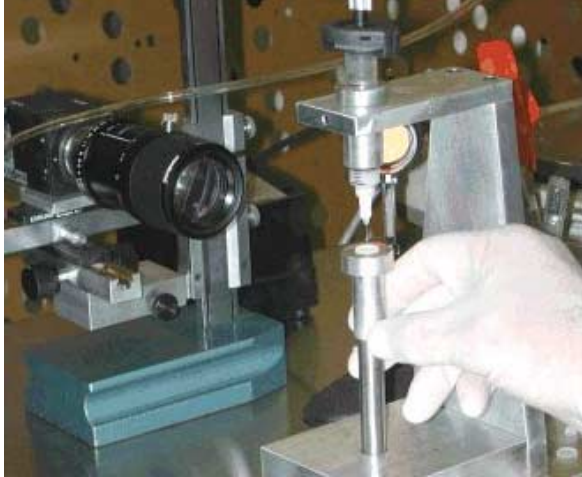
Figure 18. The adhesive was metered into 0.4 \text{ mm}^3 droplets using a fine bore needle and optical metrology.
