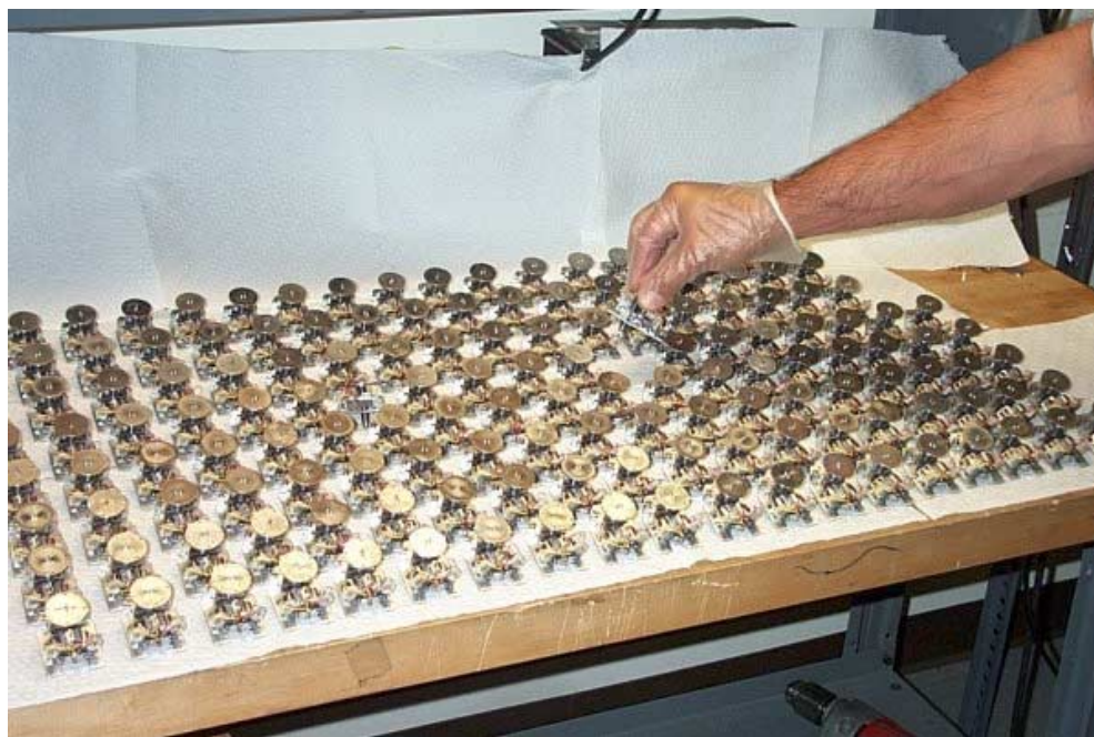
Figure 24. 186 NMSD actuators were produced and tested.
