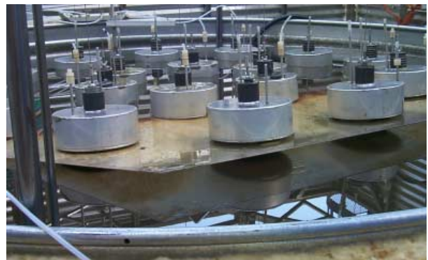
Figure 10. After floating free, the facesheet is lifted from the oil using a whiffle tree attachment to the floats. It is tilted to allow the oil to flow out.
