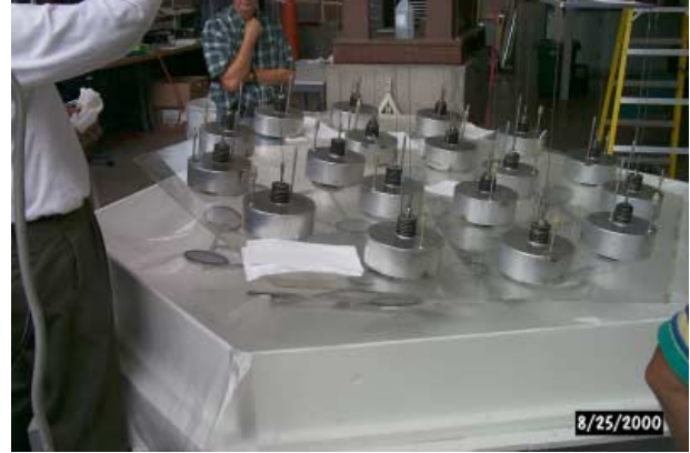
Figure 14. The facesheet was set down onto another whiffle tree.
