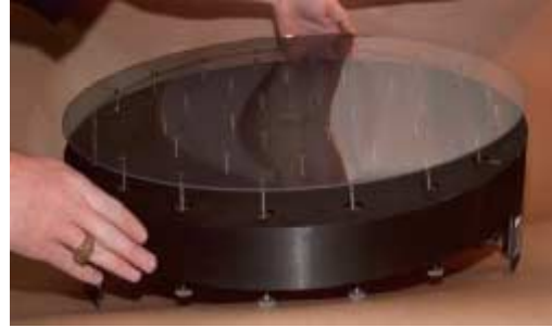
Figure 2. A prototype mirror, weighing about 20 kg/m 2 . This mirror used a 2-mm Zerodur facesheet on 36 actuators and a composite support structure.
