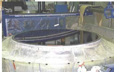
Figure 7. Fabrication of the 2-m diameter glass shell for the NGST Mirror System Demonstrator.
