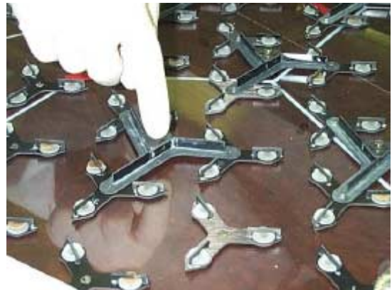
Figure 21. Attachment of loadspreader..
