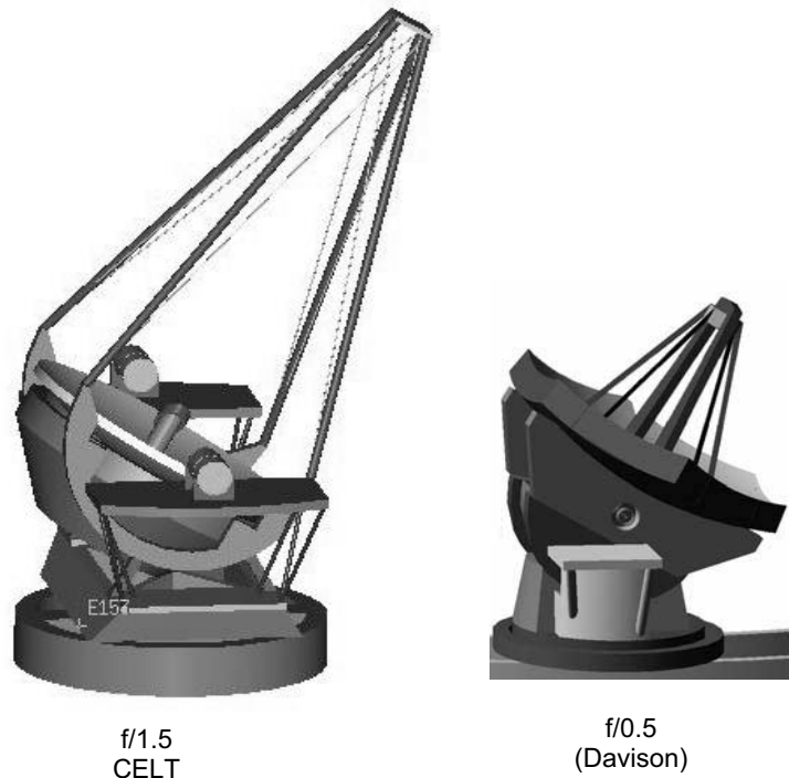
Figure 1. The difference between a telescope with f/1.5 primary and f/0.5 primary is easy to see in these two designs of 30-m telescopes.
