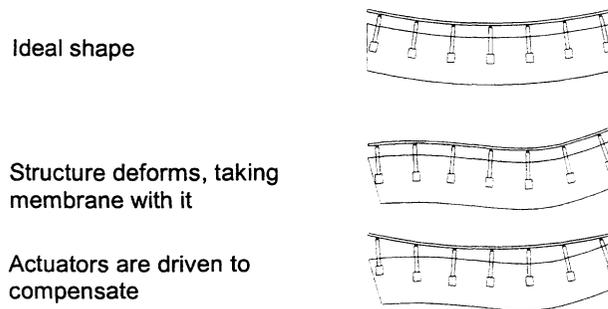
**Figure 1.** Use of position actuators to maintain the optical surface.
