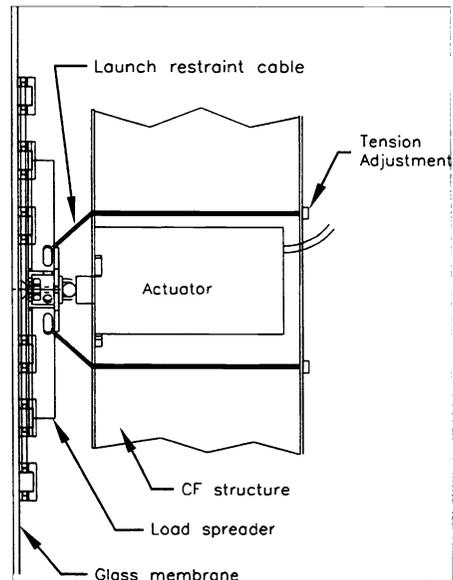
**Figure 6.** Side view showing launch restraint cables.
