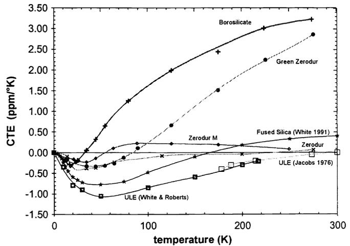
**Figure 4.** CTE for various glasses down to cryogenic temperatures.
