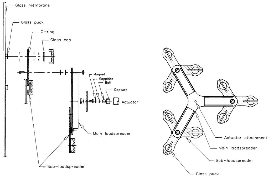
**Figure 5.** Exploded side view and assembly drawing showing the 9-point load spreaders and their attachment to the glass membrane.
