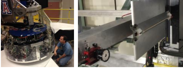
Fig. 4. Actively shape controlled 60 cm stressed lap (left) and Scanning Long-wave Optical Test System (right).
