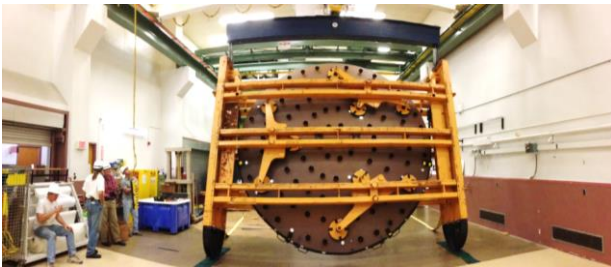
Fig. 1. The 4.2 m diameter DKIST primary mirror in the turning structure at the College of Optical Sciences, University of Arizona.
