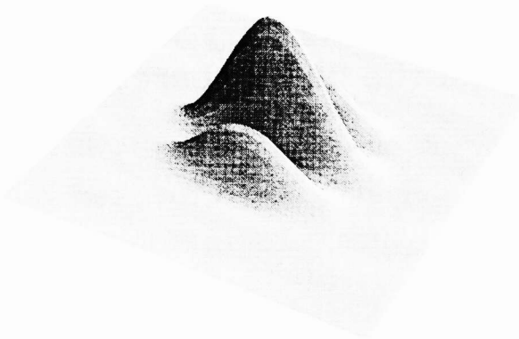
Figure 1. Surface plot of the on-axis, unaberrated PSF at the combined focus of the LBT at 4.8\mu\text{m} . The envelope of a single beam Airy pattern, 0.29 arcsec, is modulated by fringes of width, 0.069 arcsec.
