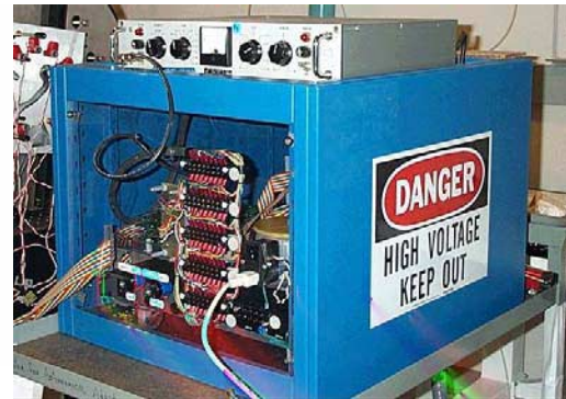
Figure 8. SMEC high voltage control system is used to pull mirror to full curvature and correct aberrations
