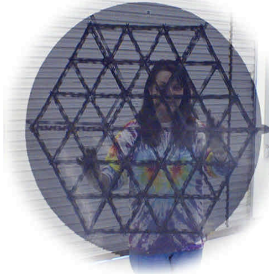
Figure 7. Lightweight reflectors built by COI demonstrate the technology for the backing structure. This mirror weighs 0.56 kg/m 2 including the mesh reflector surface.
