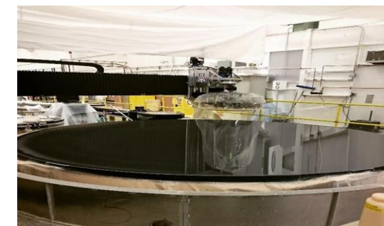
Figure 5. DKIST Primary during fine grinding phase. Surface is spectrally reflective.
