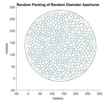
Fig. 2. A schematic of an array configuration that uses dishes with random diameters (flat distribution) ranging from 9 to 15 m in
