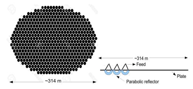
Fig. 1. A schematic of the NGAT concept showing an array of smaller dishes (left) and a cross section showing dishes co-mounted on a steerable platform (right). Image credit Arecibo Observatory.
