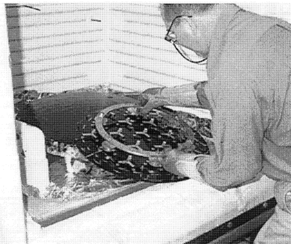
Figure 23. Deblocking the finished 1 mm thick glass membrane. The ring fixture was used for handling the mirror during deblocking and coating.
