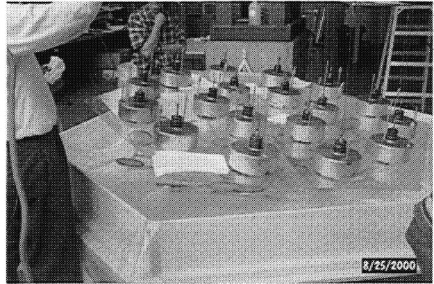
Figure 14. The membrane was set down onto another whiffle tree.
