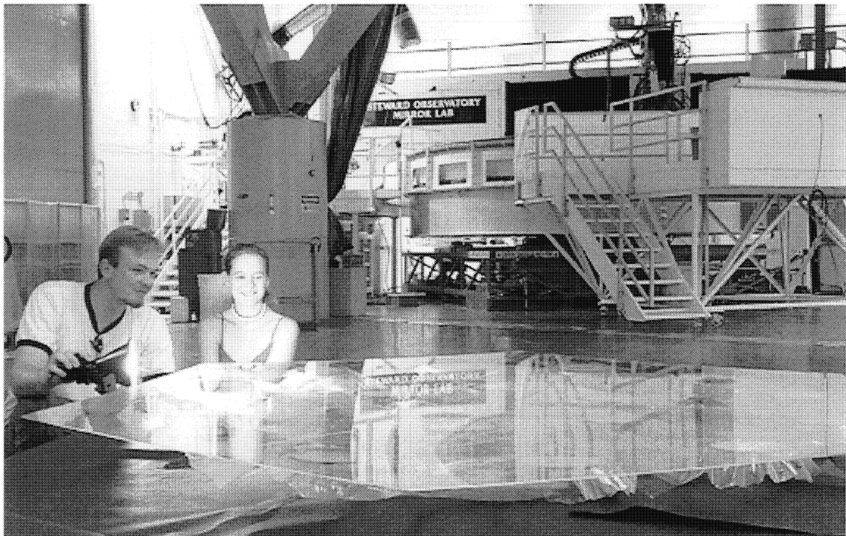
Figure 15. Completed 2 mm thick, 2-m hexagonal membrane for the NMSD mirror
