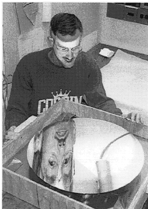
Figure 25. Glass membrane after coating with aluminum.
