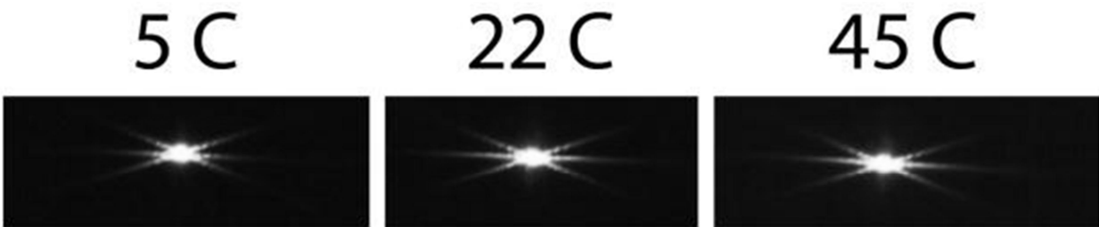
Figure 19. Bahtinov diffraction patterns over temperature with stock Al lens mount.
