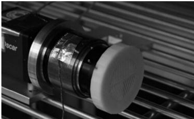
Figure 16. Leica camera lens in the thermal test oven.
