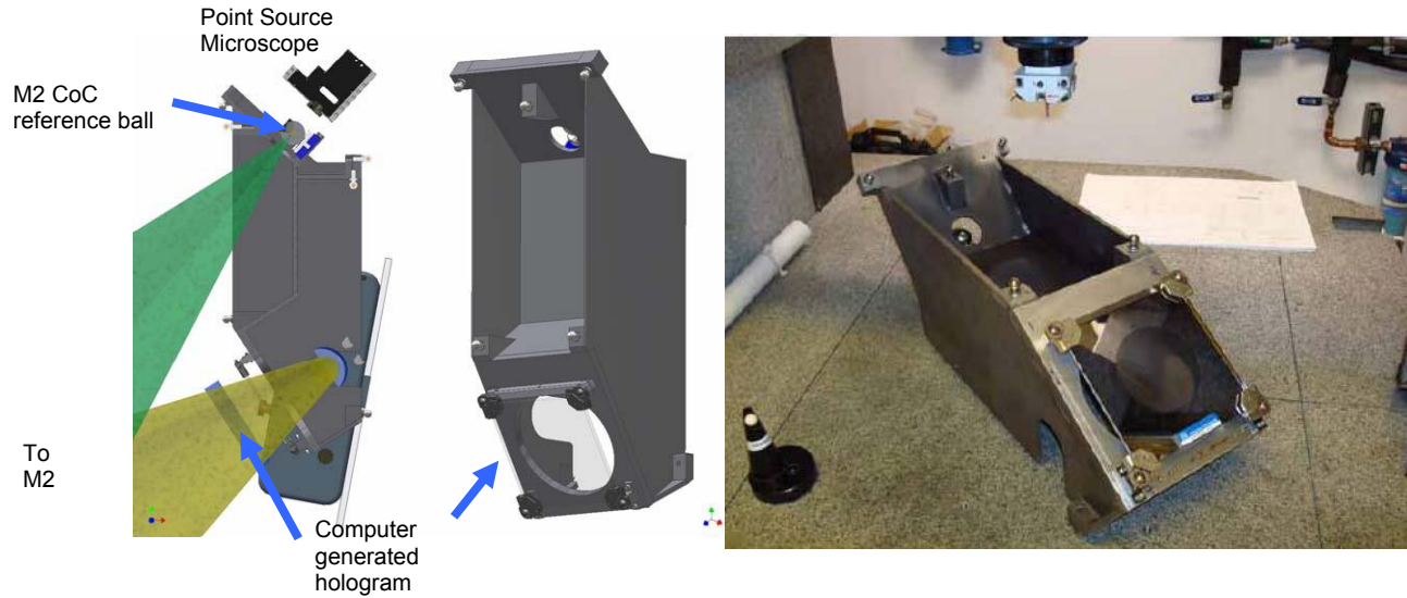
Figure 6. The invar cradle is used to provide the reference for the most critical dimensions in the optical test. The position of M2 is adjusted so that its center of curvature coincides with the M2 reference ball, which is attached to the cradle. The position of this reference ball, with respect to the CGH is controlled to < 10 \mu\text{m} over the distance of 44 cm.
