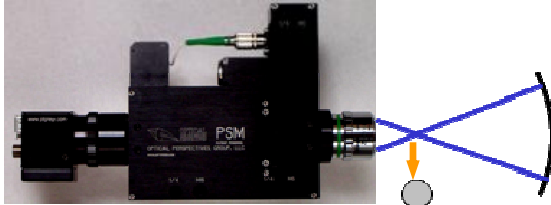
Figure 8. The Point Source Microscope is used as feedback to move M2 to place its center of curvature to coincide with the reference ball position.
