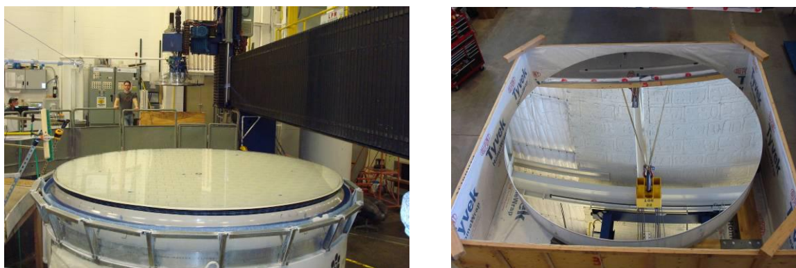
Figure 14. The 3.75 m fold sphere (M1) on the polishing machine (left) and after coating (right).
