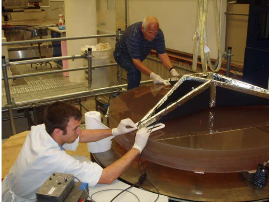
Fig. 7. The OAP curvature was measured with a custom 3-ball spherometer. The spherometer consists of a monolithic aluminum skeleton, covered with thermal insulation, that rests on 3 tooling balls near the edge of the OAP. A displacement probe at the center measures the sag to 0.3 \mu\text{m} .
