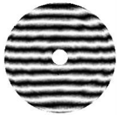
Figure 10. Interferogram, calculated from measurements for \lambda = 1 \mu\text{m} , showing the figure of the 6.5-m primary.
