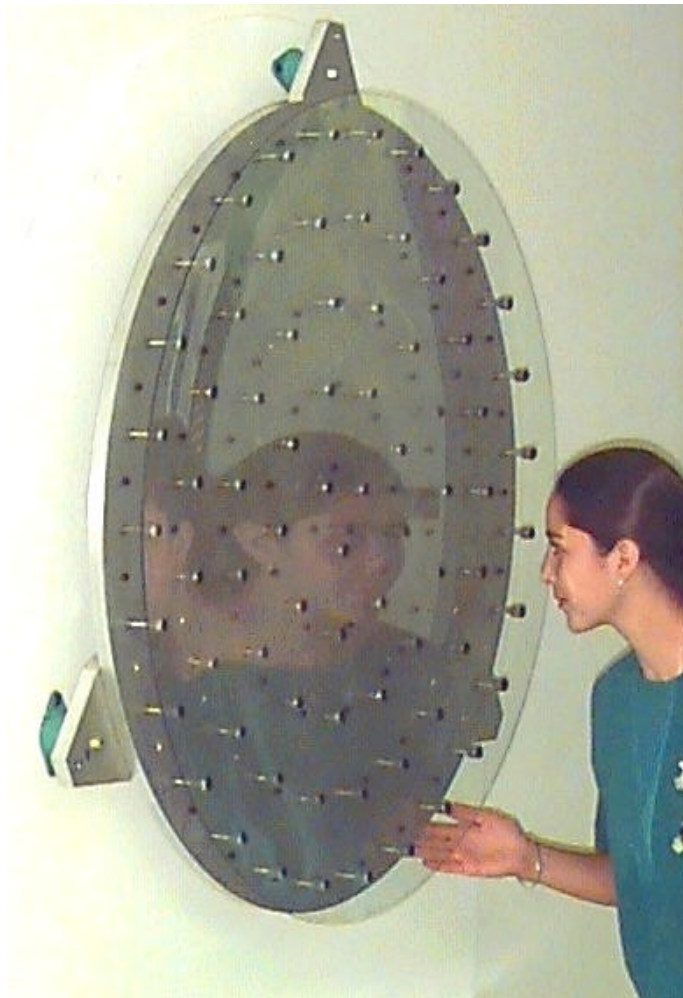
Figure 8. 1-m prototype mirror on 75 dummy actuators that survived acoustic launch testing
