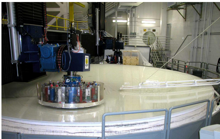
Figure 5. New 8.4 m polishing machine being used to polish the second LBT mirror. The machine has two tool carriages and can drive a variety of tools including the two 1.2 m stressed laps shown here.
