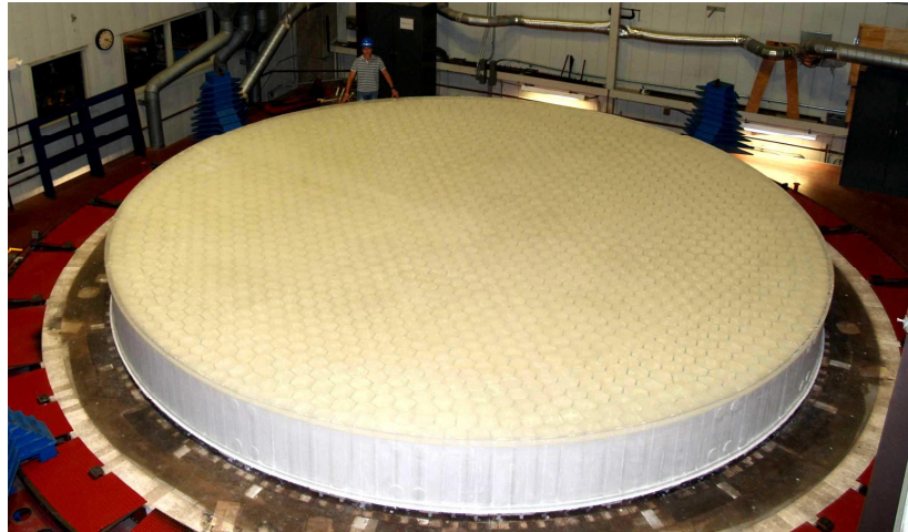
Figure 2. First GMT segment resting on the furnace hearth after a successful casting.
