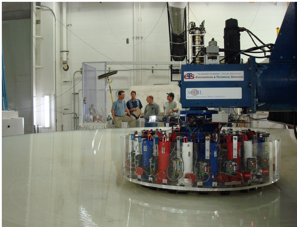
Figure 4. First day of loose-abrasive grinding the GMT segment with a 1.2 m stressed lap. This work is done on the Large Optical Generator shown in Figure 3, but converted to a polishing machine. A second 8.4 m polishing machine will be used for final figuring.
