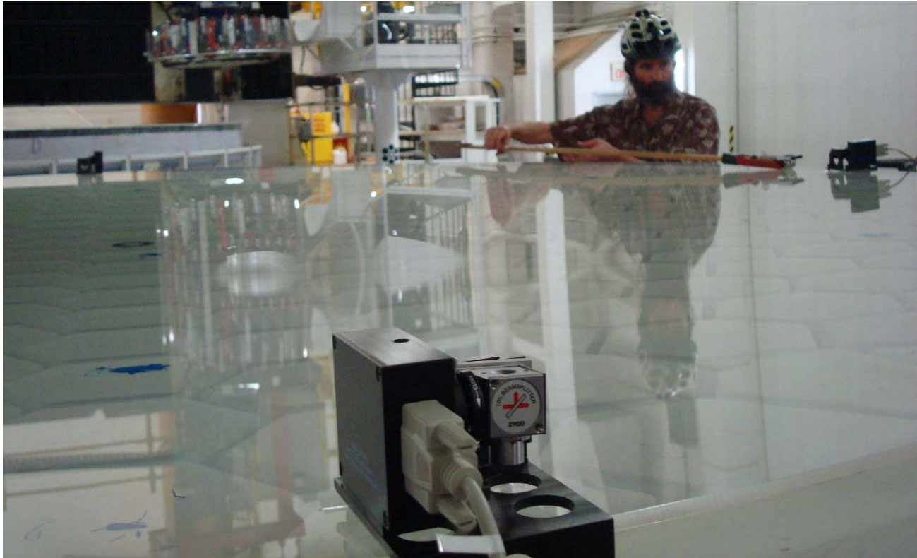
Figure 11: Testing of the 3.75 m spherical mirror with the Laser Tracker Plus system. One of the references is visible in the foreground, with two of the three other visible in the background. An optician positions the SMR mounted at the end of a wooden wand for the next measurement.
