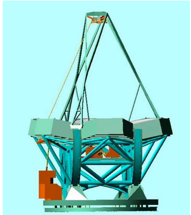
Figure 2. (Left) The AO system components mounted on the GMT telescope elevation structure (not to scale). Most of the science instruments and wavefront sensors remain fixed in place and are brought into play via a set of articulated, retractable dichroic mirrors marked low, middle and high. (Right) View showing the laser optics. Six sodium laser beacons are housed in the room on the az-platform (lower left). The beams are directed to a projector above the secondary via two flat mirrors on the elevation axis. The platform-mounted AO instruments are visible directly below the primary mirror assembly.
