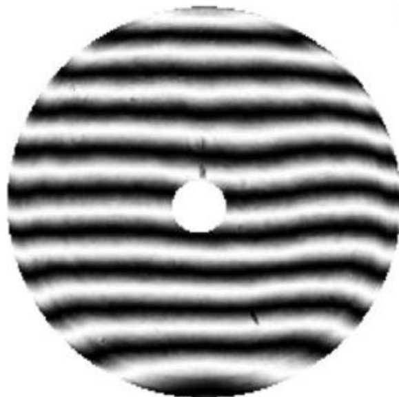
Figure 8. Measurement of the visible null lens using a CGH showing 0.035 \lambda rms error in the null lens (at 632.8 nm). The residual after removing 0.027 \lambda rms spherical aberration is 0.019 \lambda rms.
