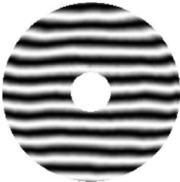
Figure 7. Measurement of the infrared null lens using a CGH, showing 0.02 \lambda rms error (at 10.6 \mu\text{m} ) in the null lens.
