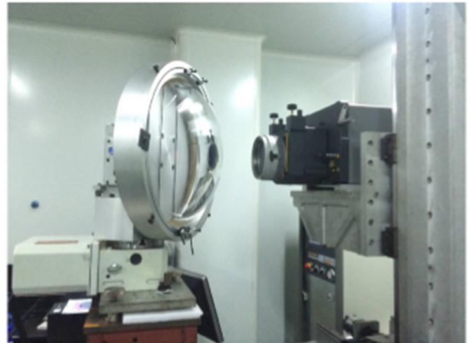
Fig. 10. Sub-aperture stitching measurement made of a large steep convex surface [32]. Image credit: S. Chen.
