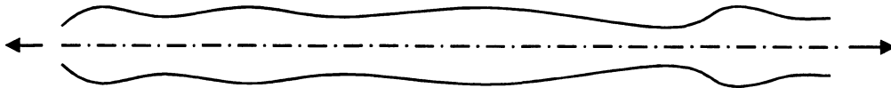
Figure 6. A membrane in tension will be flat, except for variations in material thickness.
