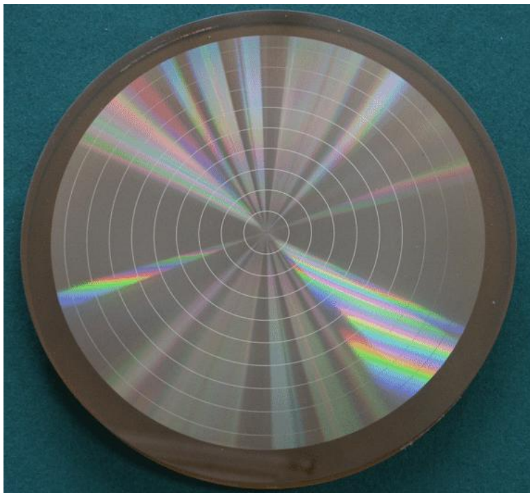
Figure 5: Photograph of fabricated CGH
