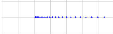
Figure 4. Spot diagram showing the camera spots that would occur in a 0 degree scan across the segment. Each division is 200 \mu\text{m} . The spot pattern is 874 \mu\text{m} across. The angular distribution of the spots is 45.9 \mu\text{rad} .
