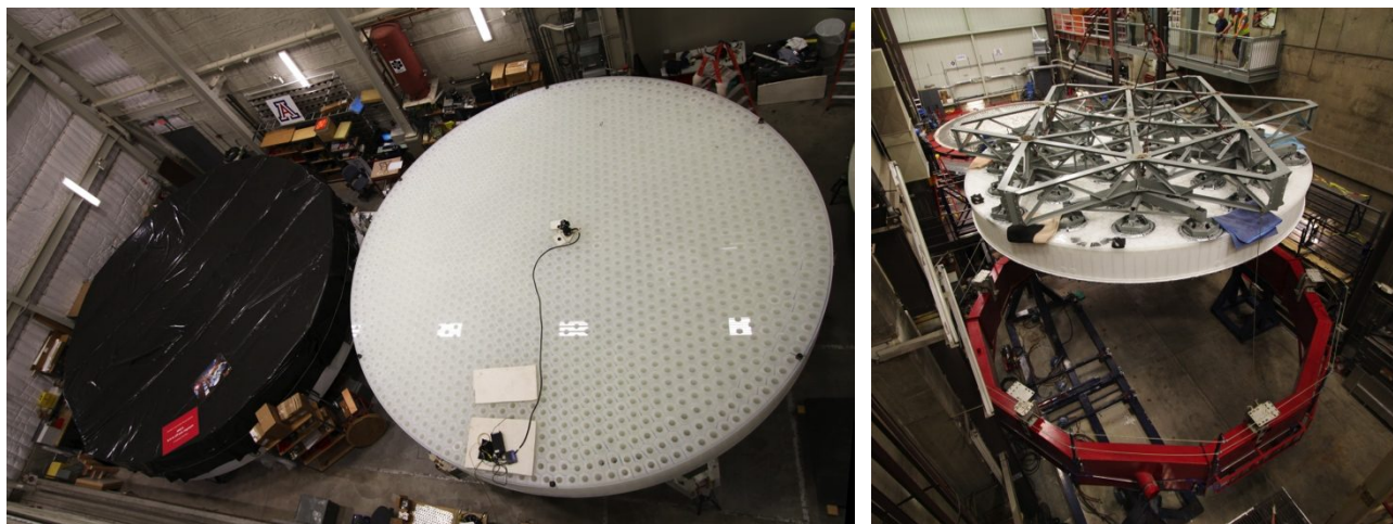
Figure 1. Left photo: GMT Segment 2 with its rear surface up in preparation for bonding of loadspreaders. A laser tracker at the center of the mirror is used to set the locations of the loadspreaders. Segment 1, with a protective cover for storage, is to the left of Segment 2. Right photo: Segment 3 being moved from the furnace to a handling ring prior to removal of the ceramic fiber mold. The mirror is lifted by a steel frame with 36 disks bonded to the mirror surface with compliant silicone adhesive. Photos by Ray Bertram.
