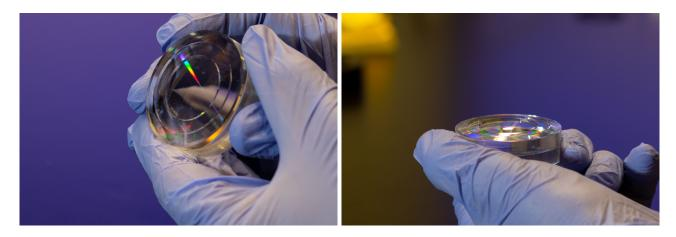
Figure 1. MODE lens prototype designed and fabricated by our University of Arizona team. This prototype has two diffractive surfaces (a front MODE surface and a traditional, single-order diffractive Frensel lens backsurface). The combination of the two diffractive surfaces and the refractive component results in a very favorable chromatic performance.
