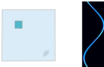
Figure 5. A sample with a small object of a different refractive index. On the right is the associated sinogram projection matrix created as the internal feature is rotated. As shown, rotation is about the axis perpendicular to the plane of the object.
