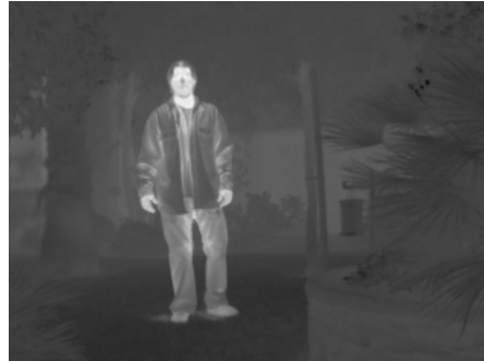
Figure 6. A picture taken by thermal imaging camera. In this picture, bright means hot. The human face appears brighter as its temperature is higher than the surroundings.
