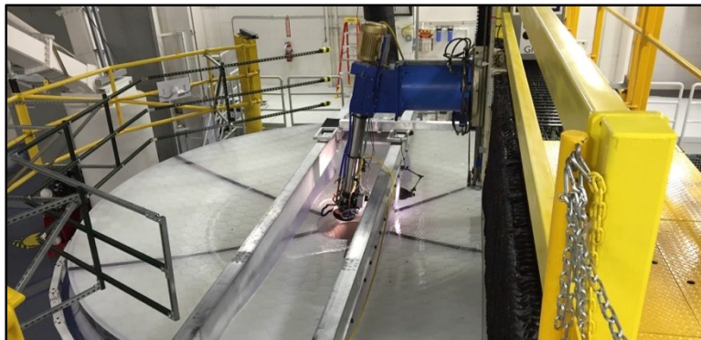
Figure 3. The 8.4-m class freeform Large Optical Generator set up for front surface generating of a 6.5-m primary mirror at the UA Richard F. Caris Mirror Lab.
