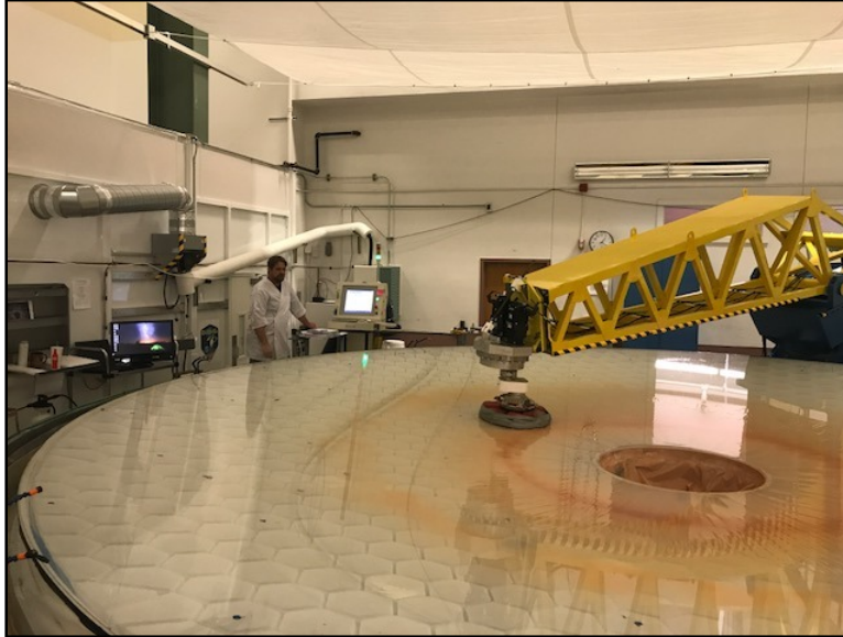
Figure 4. A 6.5-m primary mirror being polished using the computer-controlled polishing system at the UA Optical Engineering and Fabrication Facility.
