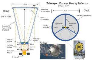
**Fig. 1.** Inflatable 20-meter Mylar balloon-based terahertz OASIS telescope concept design and configuration. [2]
