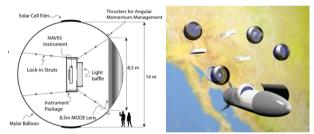
**Fig. 2.** A unit Nautilus telescope is launched in a compact configuration and inflated in orbit (left). Due to the compact launch configuration, multiple Nautilus units could be launched simultaneously in next-generation rocket fairings (right). [3, 4]
