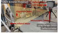
Fig. 3. 1-meter class Mylar OASIS prototype tested using the long-range deflectometry measurement setup (top-right inset).
