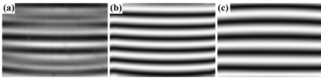
Fig. 6. Plano-concave experimental data: (a) superimposed pattern exhibiting ghost reflection; and the fringe patterns from the decoupled surfaces (b) concave (top) and (c) plano (bottom).
