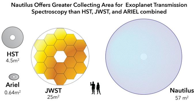
While this is not what the Nautilus mirrors will look like, this illustration shows the total collecting power of the fleet of 35 space telescopes. Each individual Nautilus mirror will, however, be able to collect more light than the Hubble Space Telescope. Credit: Nautilus team
